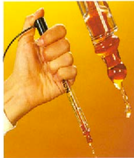
“Sure-Flow” liquid junction
